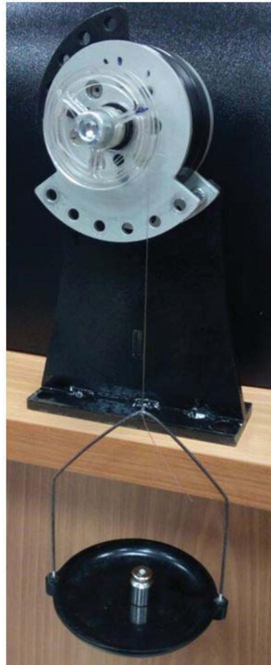
Figure 8: Installation for measuring the starting torque of the reducer with a reduction ratio of 100 using an existing method
